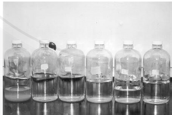
Fig. III. The blue gelatinous \text{Cu}(\text{OH})_2 precipitate from different power applied.
