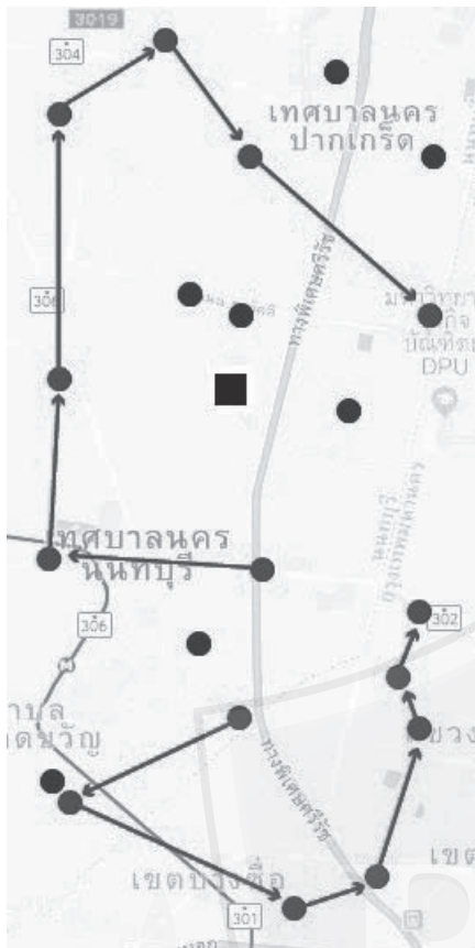
Fig. 12. Delivery route (linehaul) by proposed algorithm.
