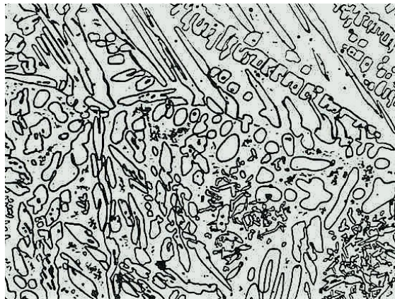
Fig. 7. As cast microstructure of duplex stainless steel showing blocks of austenite in a ferrite matrix which also contains precipitated secondary phases (Optical view x75).
