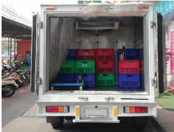
Fig. 8. Mobile cold room for keeping produce fresh and crisp
