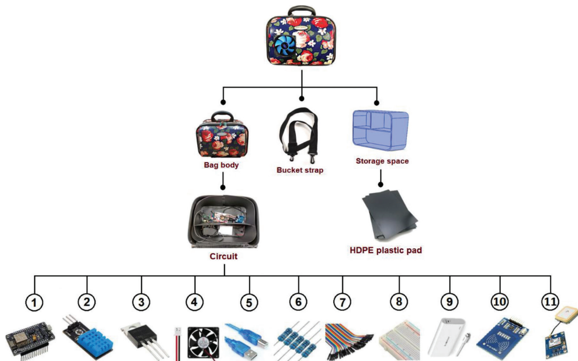
Fig. 13. System level design of the storage box
