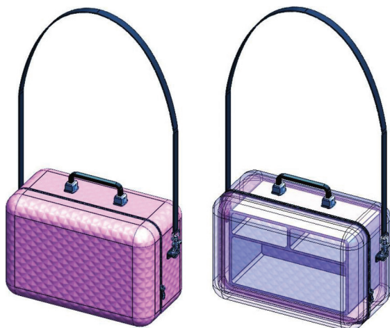
Fig. 8. Original design of “Design C” – carry-on bag inspired from classic briefcase baggage – Design B, (left) Isometric view, (right) Transparent display of isometric view
