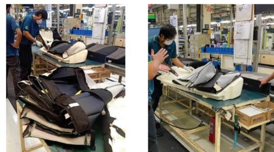
Fig. 7. Foam covering process for trims with modified listing strips.
