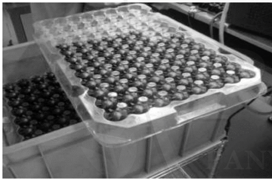
Fig. V. The improper installed position of a blower packaging box and the level of assembly table.
