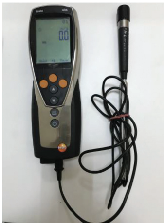
Fig. 3. Rotary vane anemometer (Testo Model 435)
