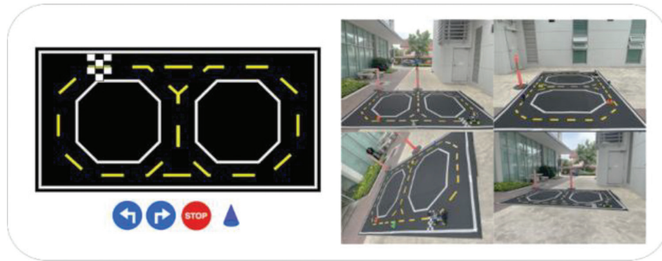
Fig. 7. The schematic diagram of the lane map site built to simulate a real driving scenario and the actual pictures taken during the experiment, as well as the markers (such as left and right turn signs, stop signs, obstacles, etc.).
