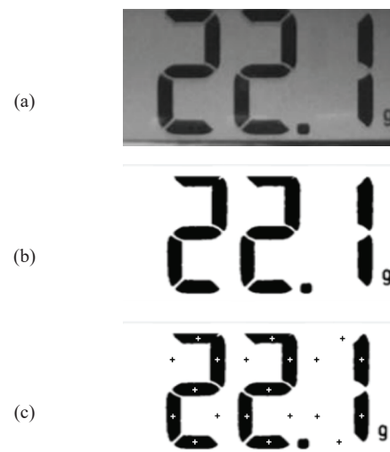
Fig. 4. The 7-Segment digit recognition process: (a) Original image of numbers from a digital scale, (b) Image converted to binary, (c) Setting the reading points of the 7 segments
