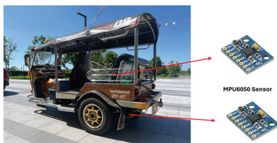
Fig. 7. The location of two MPU-6050 sensors in tricycle vehicles
