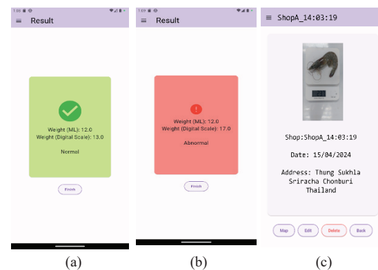
Fig. 15. The developed system: (a) Normal shrimp weight result, (b) Abnormal shrimp weight result, (c) Shrimp weight prediction history
