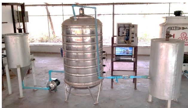
Figure 2 photo of CSTR-biogas production system combined with IOT measurement and monitoring system
