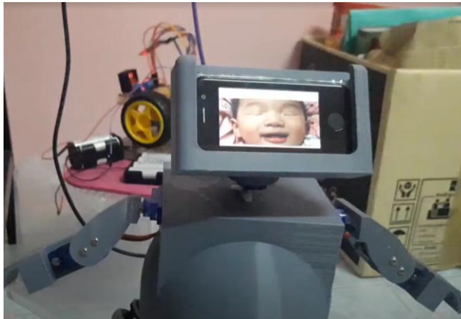
Figure 4 Voice command application on mobile for controlling motion of humanoid robot.
