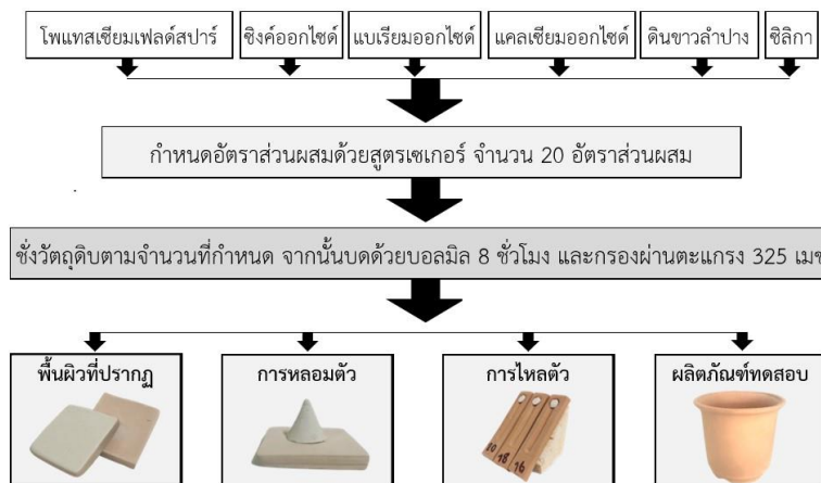
Figure 2 Preparation of specimens of copper red glaze
