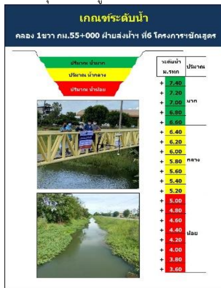
Figure 2 Control criteria for water management at canal 1 right, km. 55+000.
