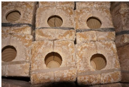
Figure 7. Characteristics of deteriorated molds that are still in daily use at the factory.
