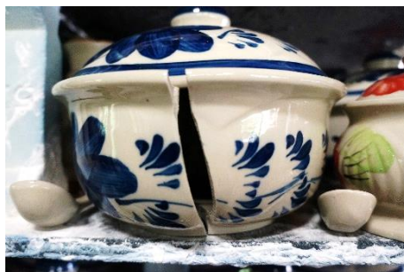
Figure 5. Characteristics of products with longitudinal cracks.
