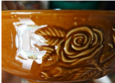
Figure 6. Characteristics of the occurrence of Pin hole defects on products formed by roller head machines.
