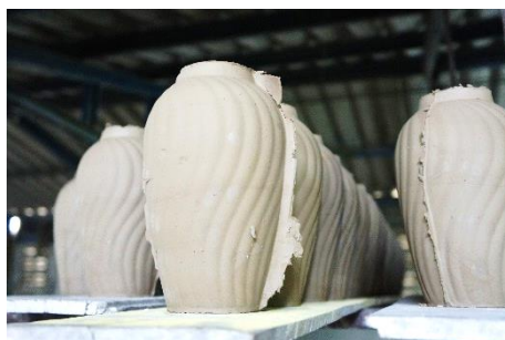
Figure 3. Products after molding with slip casting in the factory.
