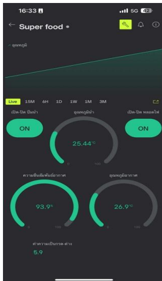
Figure 3 Displaying Results in Real-Time using the Blynk Application.
