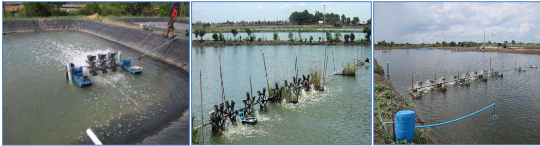
Figure 1: The propeller aerators are commonly used in aquaculture ponds.
