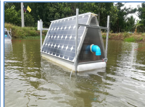
Figure 4: The implementation of autonomous oxygen generation on buoyancy for aquaculture ponds
