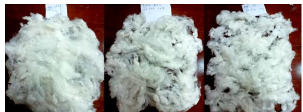
Fig. 4 : Cocoon fibers obtained from the feeder speed of 2, 3, 4 rpm
