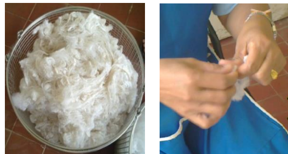
Fig. 1 : Degummed cocoons and hand crushing process
