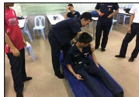
Fig. 7: Testing of system where the elderly or average person stand and sit rapidly on the mattress in a whole body fashion
