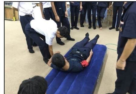
Fig. 8: Testing of alerting system where the elderly or average person stand and sit rapidly on the mattress in a whole body fashion
