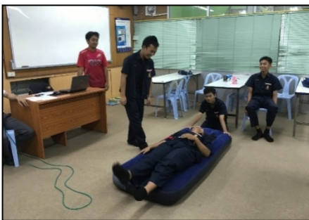
Fig. 5: Testing of alerting system where the elderly or average person stand and fall rapidly on the mattress in a whole body fashion
