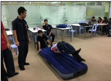
Fig. 11: Testing of alerting system where the elderly or average person stand and jump rapidly on the mattress in a whole body fashion
