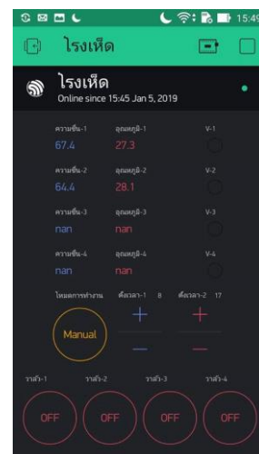
Fig. 12 The Blynk application used for controlling the IoT control box
