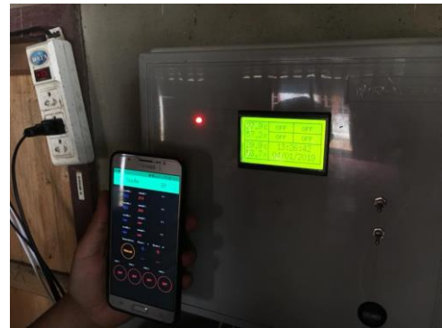
Fig. 14 Example of the second version, The IoT control box is controlling using the Blynk application installed on the smartphone
