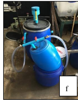
Fig. 2 Set of the 30-liter biogas-keeping barrel with the biogas-filling apparatus
