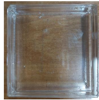
Fig. 8 Grid of transparent solar cells after polymethyl methacrylate assembly
