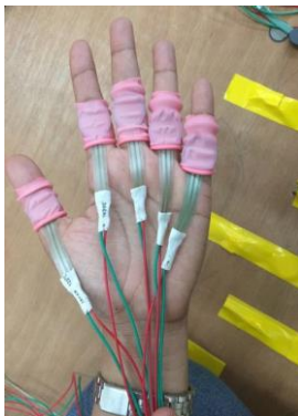
Fig. 14 Rubber finger cots with FSR sensors
