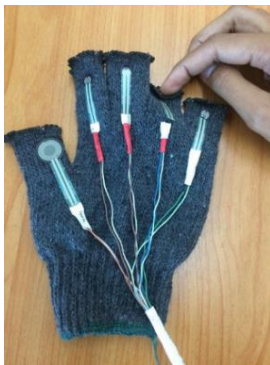
Fig. 13 sensor wiring damaged during wearing test
