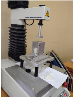
Fig. 2 Measuring cooked Konjac rice texture using rice extrusion rig
