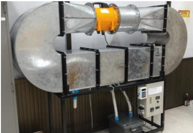
Fig. 1 The re-circulation tunnel for drying experiment
