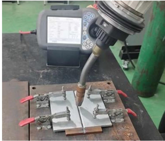
Figure 1: Experimental Setup for Clamped Workpieces in Gas Metal Arc Welding
