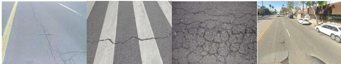
Figure 3. Four types of road damage for detection: top-left (longitudinal crack), top-right (transverse crack), bottom-left (alligator crack), and bottom-right (pothole).
