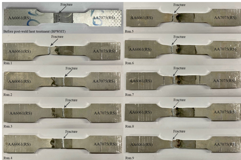
Figure 5: Tensile Fracture Locations of AA6061–AA7075 FSW Joints before and after Post-Weld Heat Treatment (PWHT) under Various Conditions.
