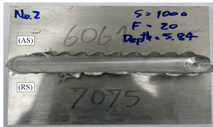
Figure 2: FSW specimen prior to PWHT, illustrating AA6061 on the advancing side (AS) and AA7075 on the retreating side (RS).
