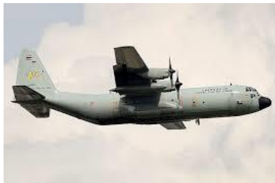
Fig. 6 C-130H with (4) T56-A-15 turboprop engines
