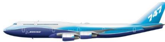
Fig. 12 B747-100 aircraft with 4 JT9D-7A turbofan engines
