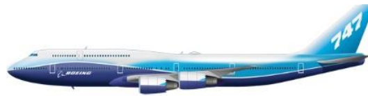
Fig. 12 B747-100 aircraft with 4 JT9D-7A turbofan engines
