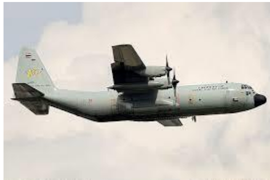
Fig. 6 C-130H with (4) T56-A-15 turboprop engines
