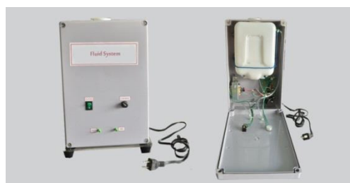
Fig. 2 Fluid system for venipuncture arm
