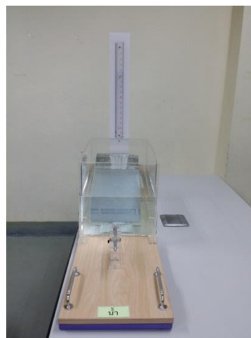
Fig.1 The simple refractive index experimental set
