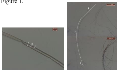
Figure 1 Fiber morphology of PALF under light microscope a) Fiber diameter (D), lumen (L), cell wall thickness (w) and b) Fiber length (L).
