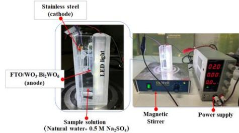
**Figure 1** Experimental setup for investigating the degradation of microorganisms utilizing the developed PEC cell.
