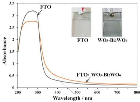
**Figure 3** The absorbance properties of composite  $\text{WO}_3\text{-Bi}_2\text{WO}_6$  immobilized on FTO substrate, as well as images of composite  $\text{WO}_3\text{-Bi}_2\text{WO}_6$  film compared to FTO substrate, are shown in the inset.
