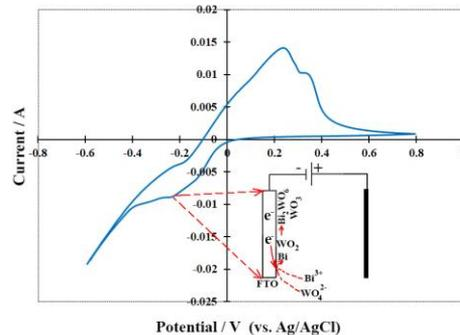
**Figure 2** Cyclic voltammogram of composite  $\text{WO}_3\text{-Bi}_2\text{WO}_6$  deposition on FTO substrate and inset of schematic reaction of composite  $\text{WO}_3\text{-Bi}_2\text{WO}_6$  film formation.
