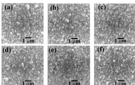
**Figure 6** SEM micrographs of composite WO<sub>3</sub>-Bi<sub>2</sub>WO<sub>6</sub> electrodes prepared at various annealing temperatures: (a) 25°C, (b) 300°C, (c) 400°C, (d) 450°C, (e) 500°C, and (f) 600°C.
