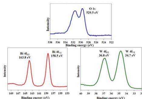
**Figure 7** XPS spectra of composite WO<sub>3</sub>-Bi<sub>2</sub>WO<sub>6</sub> electrodes prepared by cyclic voltammetry.
