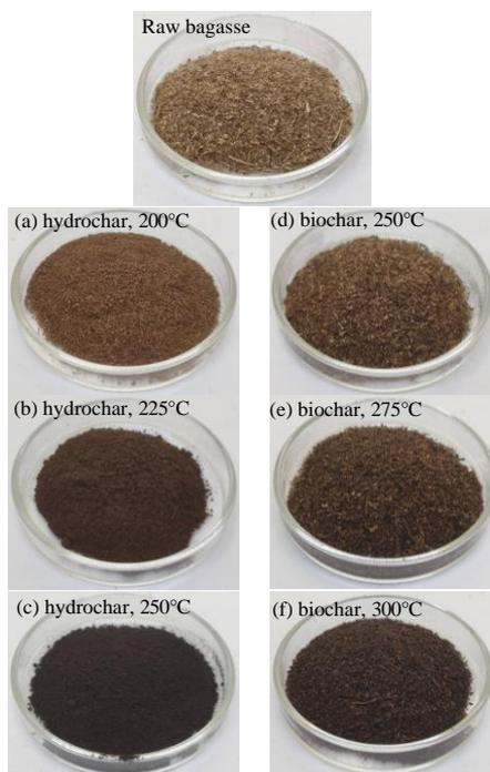
**Figure 1** Biochar and hydrochars derived from sugarcane bagasse
