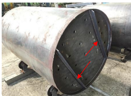
Fig. 12 Type 3- Flat Bar Type with Beams Used in Real Production in the Industrial Sector
