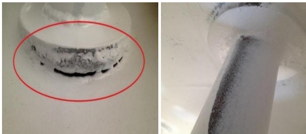
Figure 3 Defect Under the Strainer Plate
