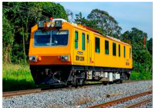
Figure 4. Track inspection Car EM120N [SRT]
