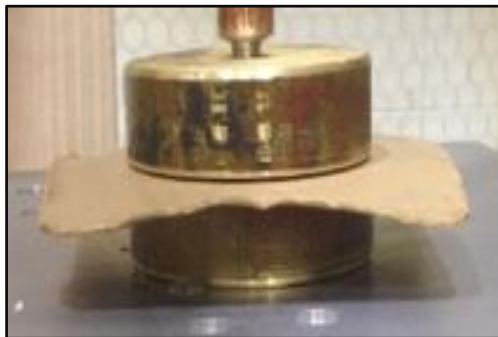
Figure 7. The experiment HV test structure consists of brass electrodes, radius 37.5 mm and the composite insulator.
