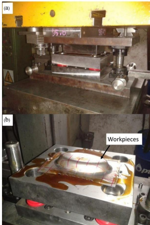
Figure 10 Deep drawing die and workpiece.
