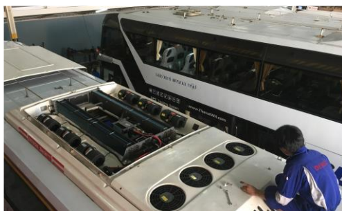
(a) Bus Air conditioner repaired.
