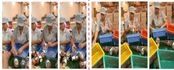
Fig. 5 Step 7 (wrap a cup with shrink film) and step 8 (fold shrink film)
