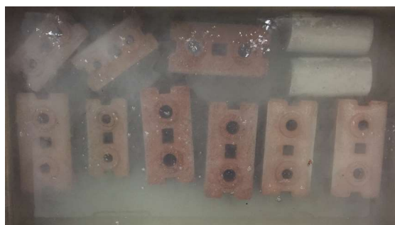
Figure 9 Immersion of CCI bricks in water
