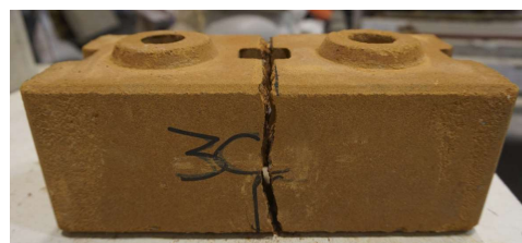
Figure 16 Typical failure of brick in splitting tensile test
