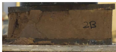
Figure 14 Typical failure of brick in compression
