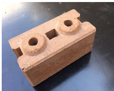
Figure 3 CCI brick sample (Region B)
