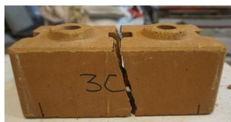
Figure 15 Typical failure of brick in flexure
