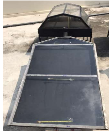
Fig. 5 The completed mixed solar dryer
