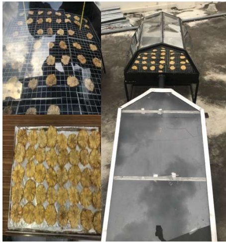
Fig. 4 drying of pineapple in the solar dryer cabinet
