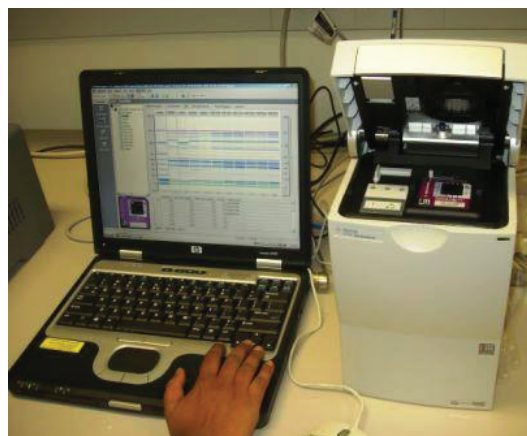
Figure 5. Equipment for capillary electrophoresis, suitable for proteins extracted from crushed grains of either wheat or rice. The resulting protein patterns can be seen on the computer screen.
