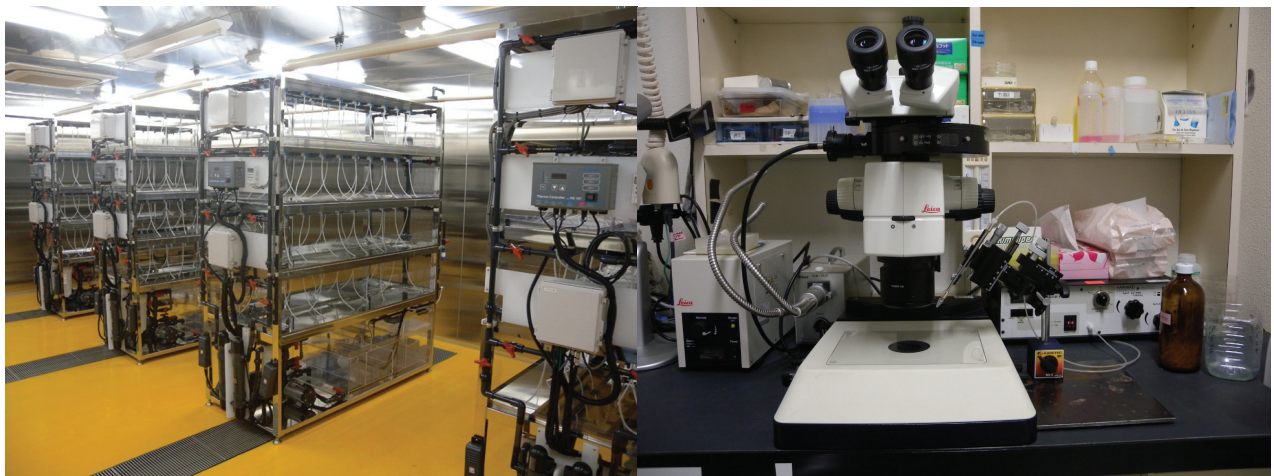
Figure 2. Fish facility (left) and microinjection apparatus (right) for visiting researchers in NBRP Medaka. Users have access to their own fish racks during their stay at NIBB. Fish caretakers and lab technicians assist with screening of the TILLING library, constructing sgRNA plasmids for CRISPR-Cas9 genome editing and microinjecting eggs.
