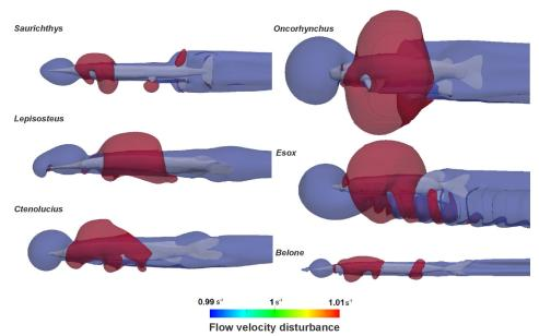
**Figure 3.** Flow velocity disturbance around the models of *Saurichthys*, *Lepisosteus*, *Ctenolucius*, *Oncorhynchus*, *Esox* and *Belone* at 1 ms<sup>-1</sup> inlet velocity. Modeling at different velocities shows that the speed-dependent variation of flow disturbance is nearly negligeable. Fish models are not to the same scale (after Kogan *et al.*, 2015).
