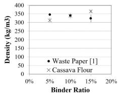
Fig. 4 Density of sawdust briquette
