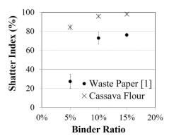
Fig. 5 Shatter index of sawdust briquette
