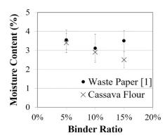
Fig. 3 Moisture content of sawdust briquette
