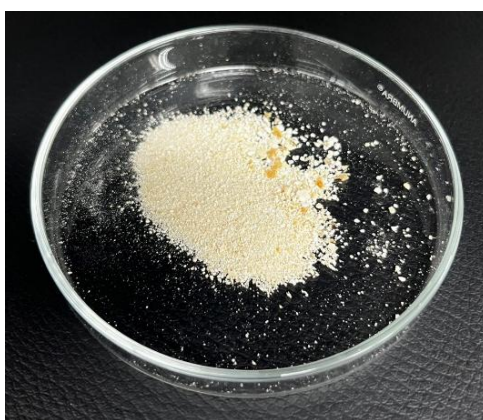
Figure 3 Crude bromelain powder from stem residue waste by using freeze drying technology.
