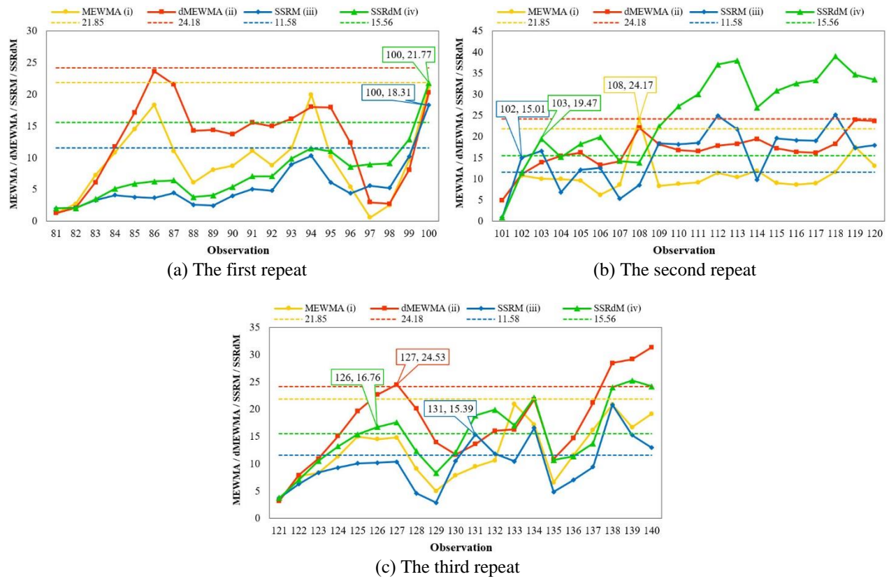
Figure 12 UCLs and control statistics in Phases 1 and 2 of the (i), (ii), (iii), and (iv) control charts for detecting of three variables of the blade wheel of blower for a non-normally distributed process under \lambda = 0.5 and \delta = 0.25
